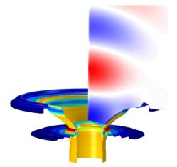
With vibroacoustic simulations explanations can be found for dips and peaks in the frequency response, and the simulations can be for virtual prototyping where solution proposals can quickly be tried out.
